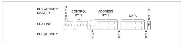
FIGURE 6-2: SRAM/RTCC SEQUENTIAL WRITE
