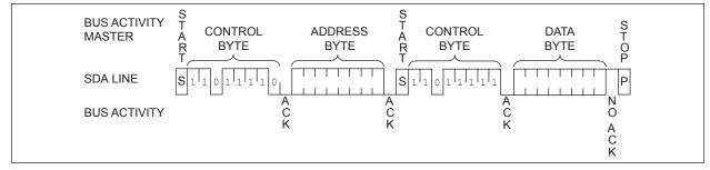
FIGURE 6-5: SRAM/RTCC SEQUENTIAL READ
